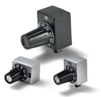
Miniature adjustment knob MF with 50th graduation, revolution counter (to 10 rev.), locking mechanism and cardan coupling
