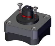
Recommendation for mounting screws: 4-40 x 1/4" Max. allowed tightening torque 0.67 Nm.
