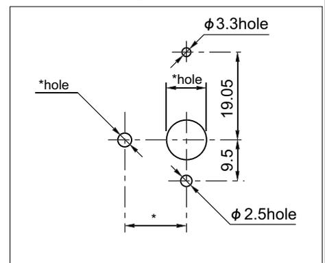
Note: The diameter of \*hole is depending on the diameter of potentiometer to be mounted.
