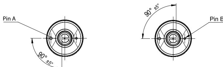
**Signal definition for custom rotation angles (without mechanical stop)**
