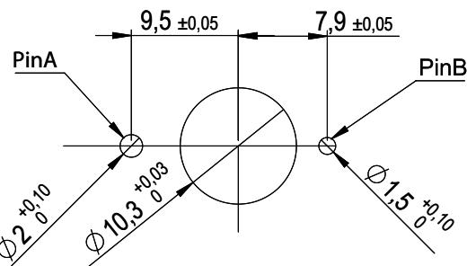
Either pin A or pin B must be chosen as anti-rotation pin. Please select by specifying the variant in the order code. The unused pin can be left out when drilling.
