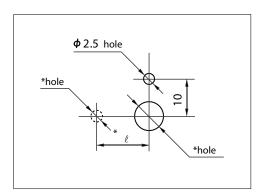
Note: The diameter of \*hole is depending on the diameter of potentiometer to be mounted
